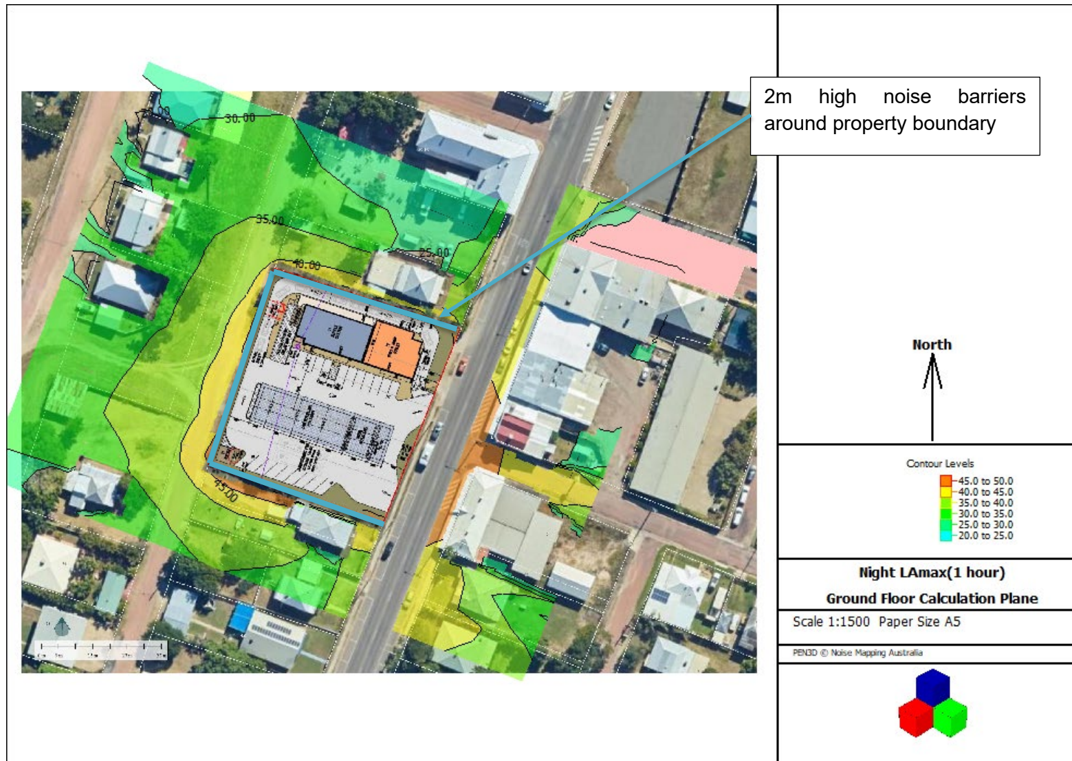
Figure 4: L Amax (60 min) Night Noise Levels from Operations All Sources Excluding Waste Truck and Delivery – Ground Floor (with 2m Property Boundary Barriers)
